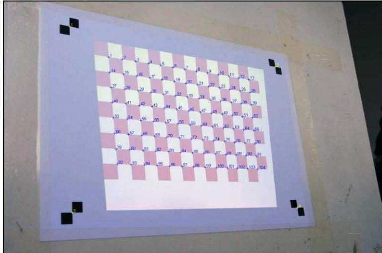
Figure 1: Typical image for camera–projector system calibration.
