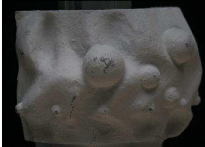
Figure 2. Calibration unit used for identifying relations between coordinate systems.
