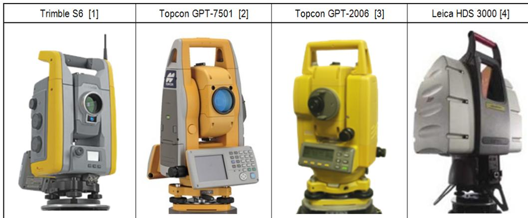
Figure 1: Used instruments
