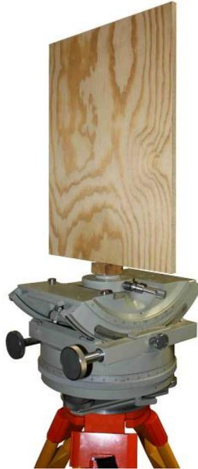
Figure 2: A target wooden board fixed onto the photogrammetric camera carrier and placed on a surveyor's tripod
