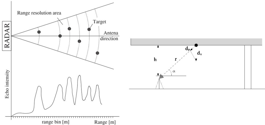
Figure 1: Radar range resolution principle (left) and radial displacement and projected displacement (right)
