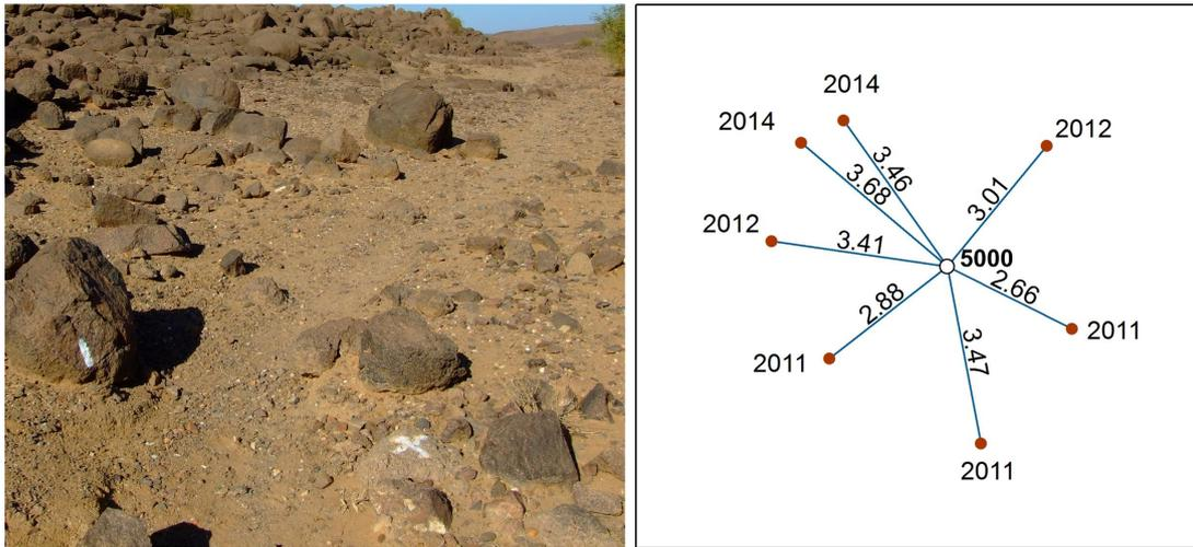
Figure 7: The initial point 5000 of the local coordinate control network (left). The control measurements on point 5000 during the archaeological seasons 2011, 2012 and 2014. The calculated distances are in cm (right).
