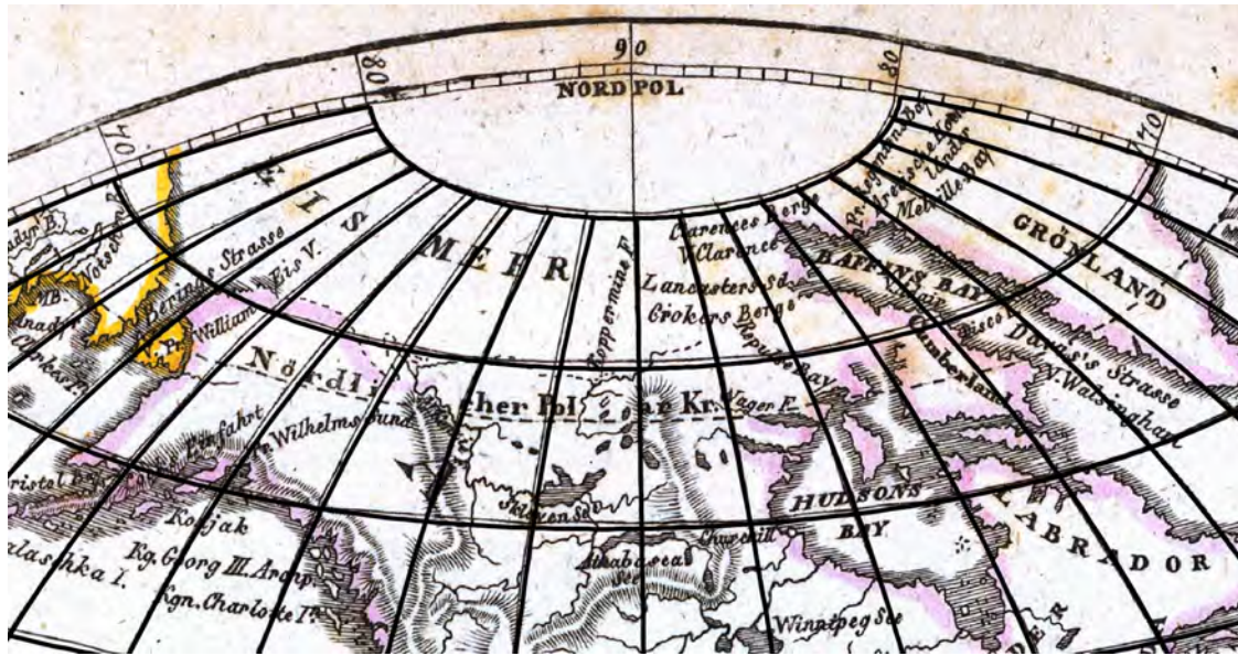
Figure 16: The map graticule reconstructed from the determined parameters. Small residuals are obvious if the analyzed map rotation \alpha = 1.7^\circ is involved (source: [3]).
