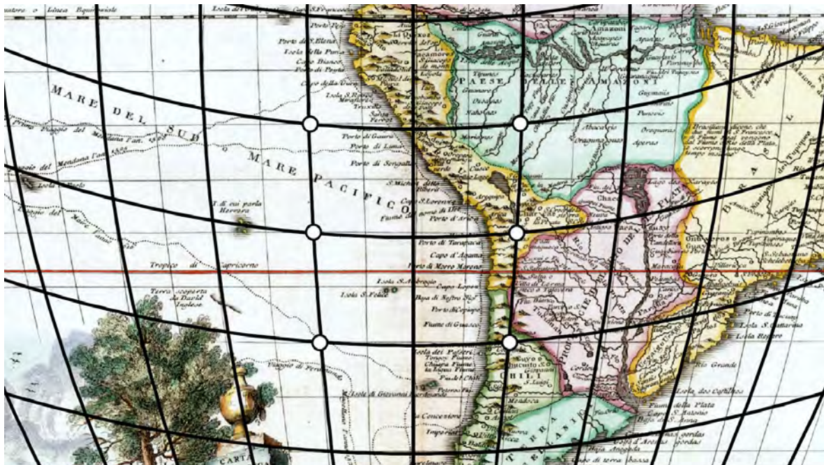
Figure 8: Insufficient amount of analyzed features on parallels (inappropriate grasp of their shape) lead to the detection of the different projection (source: [3]).
