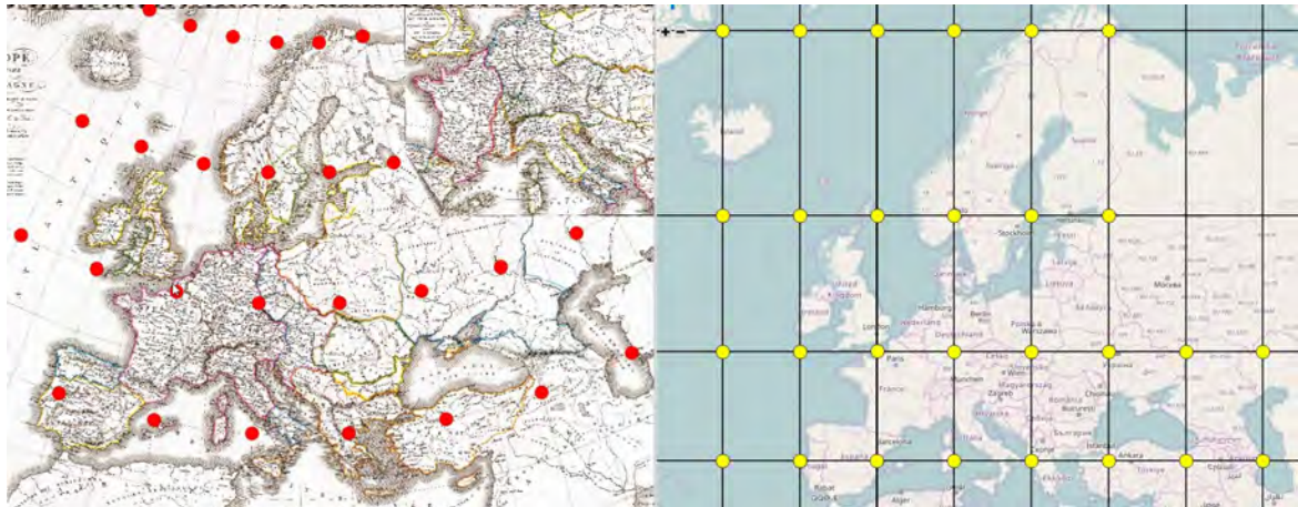
Figure 12: The set of control points on the analyzed and reference maps represented by the intersections meridians and parallels acquired in detectproj software.
