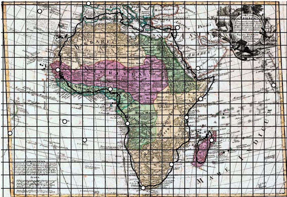
Figure 3: Georeferencing of a small-scale map in Bonne projection to the destination coordinate system in the Mercator projection using the similarity transformation.
