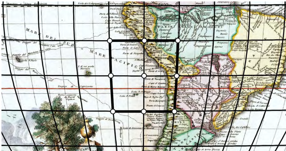
Figure 9: The analyzed features covering a small part of the analyzed territory; the estimated graticule fits into the original only inside the convex hull. Bonne projection, \varphi_1 \neq 0^\circ , instead of sinusoidal is detected (source: [3]).
