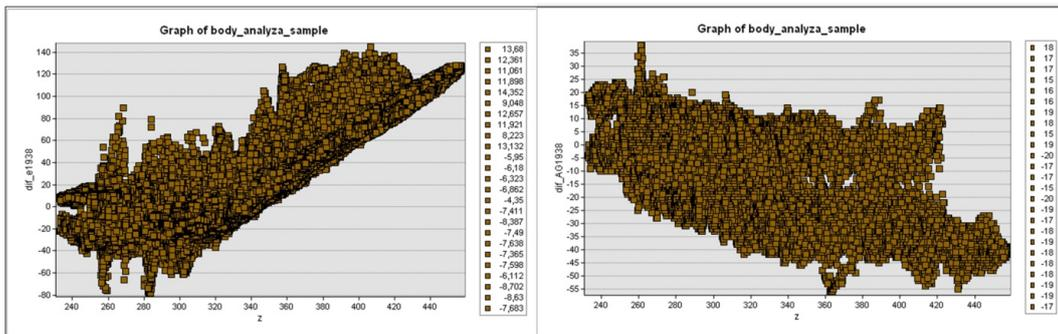
Figure 9: Graph of dependence of the estimated elevation error on the etalon data – year 1938. DSM computed by LPS (left), by PhotoScan (right). All elevation values are in meters.
