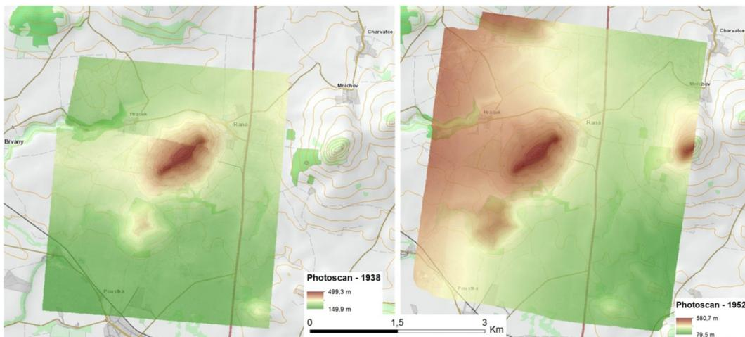
Figure 6: DSM derived from aerial photographs (1938 and 1953) using Agisoft PhotoScan
