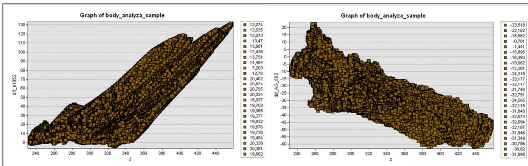
Figure 10: Graph of dependence of the estimated elevation error on the etalon data – year 1953. DSM computed by LPS (left), by PhotoScan (right). All elevation values are in meters.
