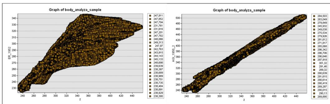
Figure 8: Graph of dependence of the estimated elevation on the etalon data – year 1953. DSM computed by LPS (left), by PhotoScan (right). All elevation values are in meters.
