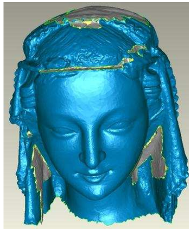
Figure 5: Surfaces filled in from the CT data (grey) to the LORS data (blue) in unreachable areas for LORS
