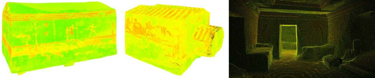
Figure 3: Typical range-based point clouds acquired with a TOF laser scanner, visualized in color-code mode.
