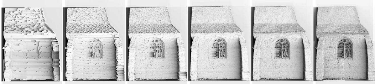
Figure 2: Example of the pyramid approach results for surface reconstruction during the multi-scale matching.
