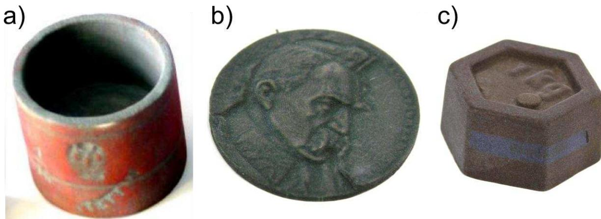
Figure 15. Printed copies of the measured objects: a) volume reference cup; b) occasional medal; c) weight reference.
