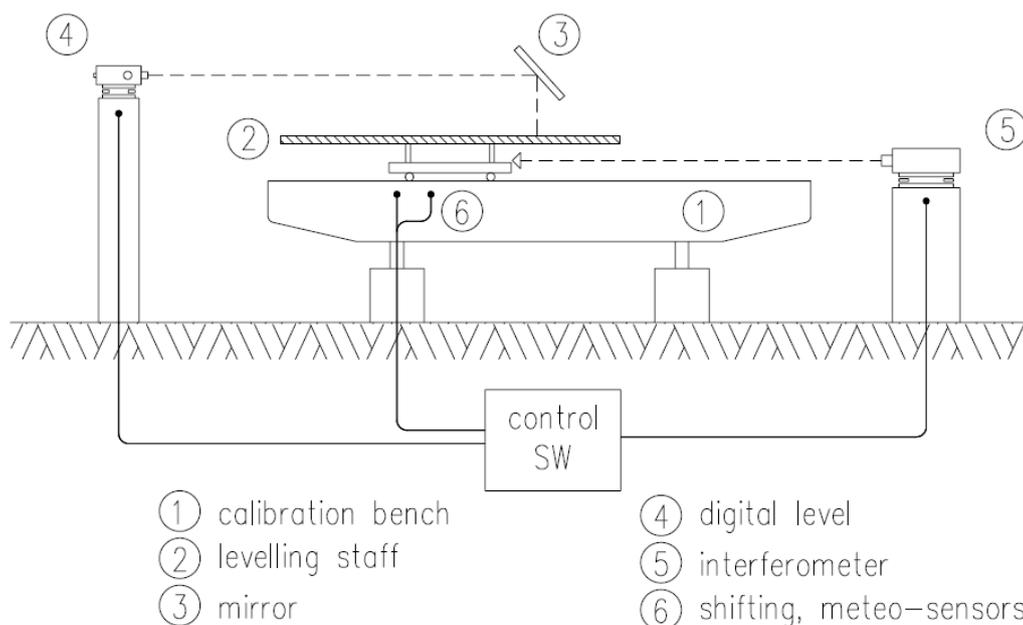
Figure 1: Scheme of horizontal comparator for system calibration
