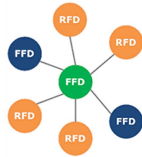
Figure 3. ZigBee star topology (FFD – fully functioning device – coordinator, FFD – fully functioning device, RFD - reduced function device)
