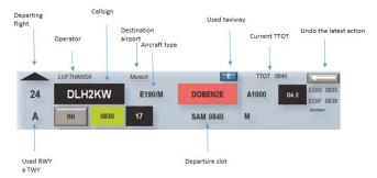
Figure 1. Electronic flight strip.
