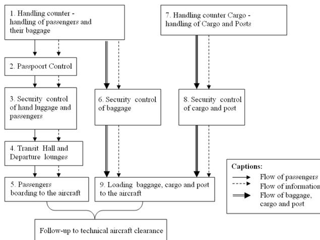
Figure 1. Block diagram of the traffic handling [2]
