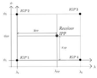
Figure 3. Principle of interpolation of the IPPs.
