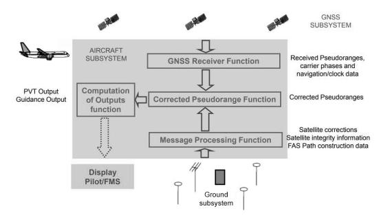
Figure 5. Data processing scheme of GBAS avionics.
