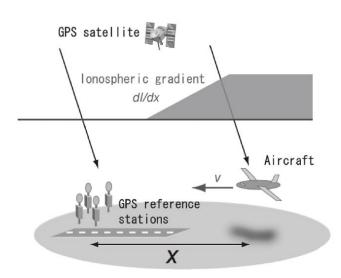
Figure 4. Spatial ionospheric delay gradient.
