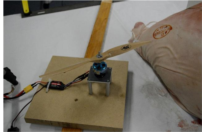
**Figure 1.** The mechanism with wooden propeller and Hobby king 910 kV engine.
