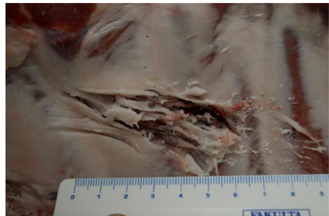
**Figure 3.** The hard tissues injury caused by Emax 650 kV engine with plastic propeller 13/4.5".
