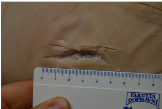
**Figure 2.** The soft tissue injury caused by DJI 400 kV engine with plastic propeller 15/5.2".
