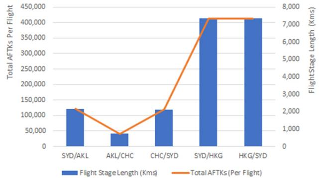
**Figure 13.** The relationship between flight stage length and AFTKs produced on the Qantas Freight Boeing B767-300 freighter services
