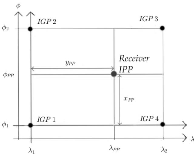
Figure 3. Principle of interpolation of the IPPs.
