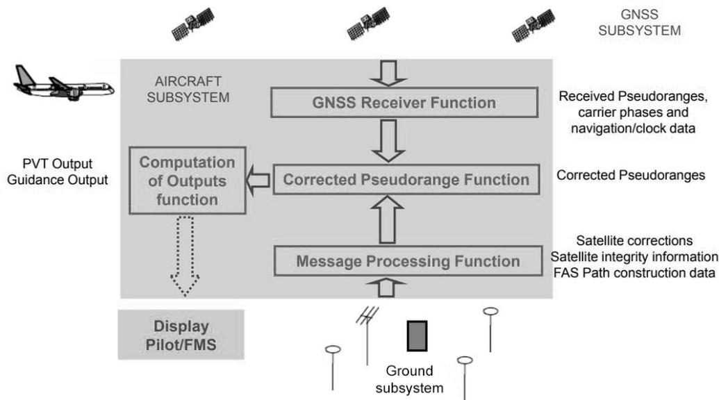
Figure 5. Data processing scheme of GBAS avionics.
