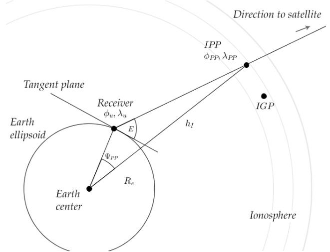
**Figure 1.** Principle of the IPP (Ionospheric Pierce Point).
