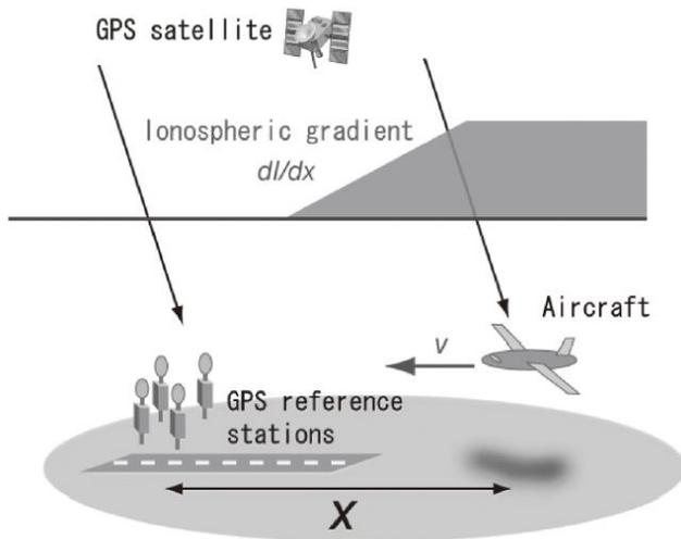
Figure 4. Spatial ionospheric delay gradient.
